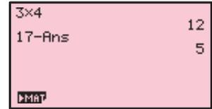
If you start an expression with an operator such as **+**, **=**, etc, the previous answer Ans is automatically inserted ahead of the operator. For example, the previous answer can be halved simply by pressing **÷**  $2$  **EXE**.
